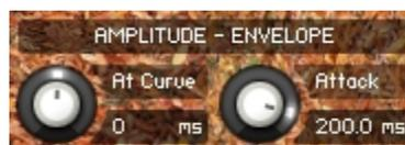
The **At Curve** knob adjusts the curve shape of the attack phase. A value of zero results in a linear curve, negative values make the shape more concave, and positive values make it more convex.
